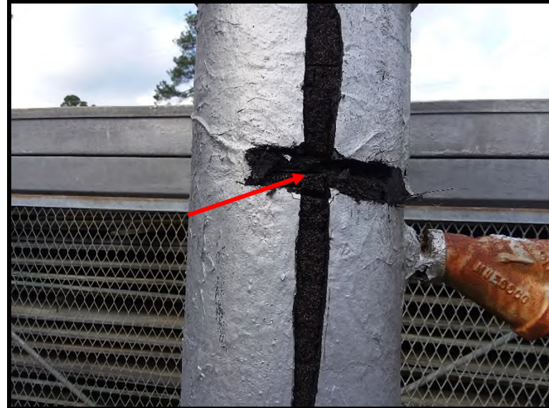
6 The black mastic located between the joints of the sulfur rock insulation tested positive for asbestos (4% chrysotile).
